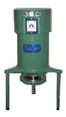
Features: Follow by Japan Foundrymen's Society (NIK) standard, this apparatus is to determine the remaining dry mass after a drying process of the original matter which is previously weighted. It provides a fast moisture measurement.
