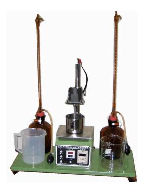
Features: The tester is to determine the amount of active bentonite clay present in the sand.
